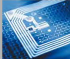
The abbreviation RFID (Radio Frequency Identification Application) stands for an innovative technology that allows products to be identified by radio waves. Instead of optical bar codes, minute chips are used. PACO R & D has been continually developing PACO screen cloths to increase the minimization of RFID chips.
