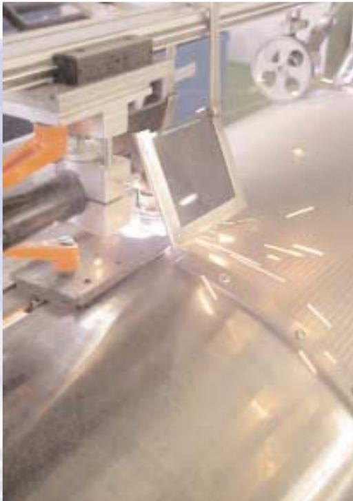
Unit for plasma-cutting PACO-Autoscreen-mesh preventing from unravelling in the later processes.
