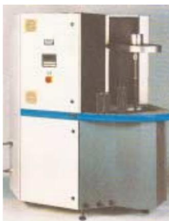
"Clean it, don't trash it" is the motto of the "Two-mode" ultrasonic cleaner with hot fluid flushing made by Bodensohn Präzision, Seligenstadt, Germany. After just three minutes of cleaning, a PACO metal filter from a diesel engine is 100% fit for re-use.
