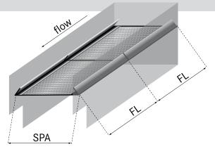
Typical screen fixations for side tensioning
