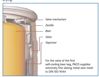
PACO as "Infinite" Innovation Partner A particular strength of certain zeolites is that there is almost no limit to the amount of times that they can absorb water and release it again, when heated – a characteristic fundamental for the economic use of ZEO-TECH. In the case of the party beer keg, ZEO-TECH is put into practice by using a multi-walled container with cavities filled with either a zeolite-crystal in a vacuum or with a water-soaked
